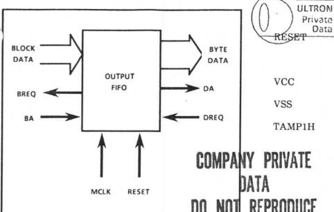
(U) The Crypto-Engine™ is a 68-Pin Grid Array device. The data path channels are organized to permit good red-black separation and operate using asynchronous control signals. This permits the maximum performance interface to the Crypto-Engine".
